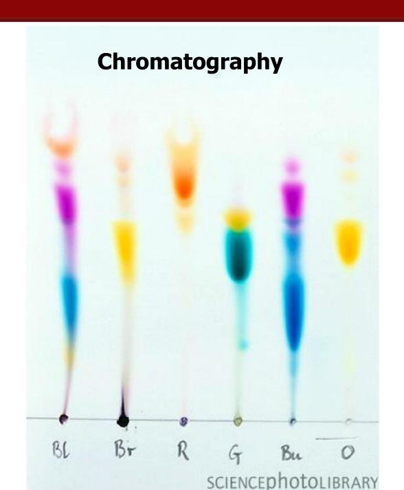
**Chromatography** – separation of a mixture into individual components
