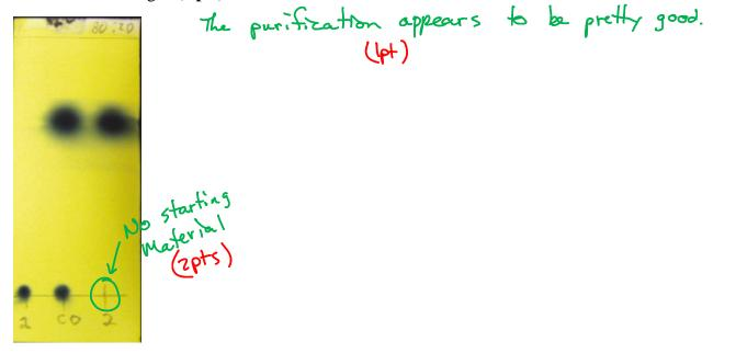
h) Calculate the R<sub>f</sub> value of the starting material and the product of the reaction. What is the cause of the lower R<sub>f</sub> value for the leftmost spot? (4 pts)
