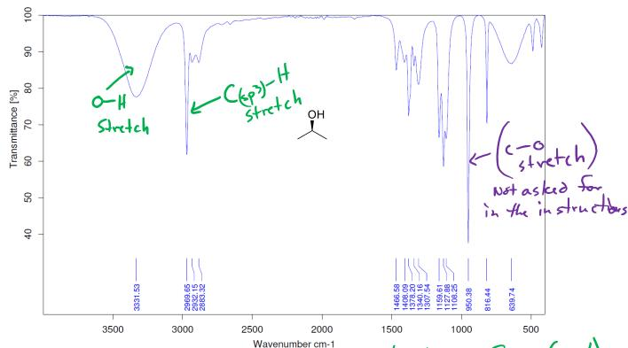
Since the O-H stretch is broad and at lower freq. (cm-1), the sample has sufficient concentration to be H-bonded. No evidence of a free O-H stretch is present as would be expected in the gas-phase or dilute solution. See Section 12.40 in London.
