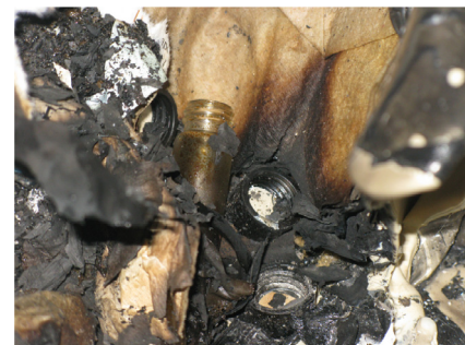
Figure 11. Catalyst fire inside trash receptacle.
