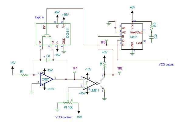
You will construct and test this circuit in sections in order to minimize mistakes and see the functionality of each section. Start by building the integrator. Use a 1 M $\Omega$  resistor and a 10  $\mu$ F capacitor. This will provide a long enough time constant so you can easily see the charging with the scope or DVM.
