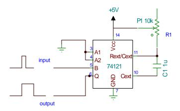
Hook up the circuit shown above. Start with C=1.0 microfarad and use a 10 K potentiometer for P1. Use the square-wave output from your relaxation oscillator to trigger the one-shot. Trigger the oscilloscope from the input trigger, and look at the output of the one-shot on the scope. Vary the value of R1 by turning the knob on the potentiometer, and you should see the "stretched" output pulse vary in duration.
