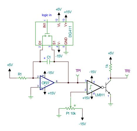
Set the threshold at -5V. Monitor test point 1 and 2 simultaneously so you can look at the response of the comparator as the integrator is working. You still have control of the reset with the switch. Change the threshold to -10 V. Be sure you understand how your circuit is working at this point. When you are convinced that your circuit is working properly, speed up the integration by replacing the 10  $\mu$ F capacitor with a 0.1  $\mu$ F capacitor.
