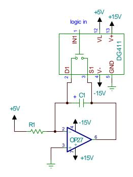
Test the reset of your integrator. What input is required at IN1 to "integrate" and what input is required to "reset"?
