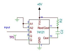
Confirm that the one shot fires on the rising edge of the input pulse. Change the capacitor to 1  $\mu$ F and the resistor to 10 K to shorten the pulse. Add the one shot to your circuit so that the comparator controls the one shot and the one shot resets the integrator. Look at the output on pin 6 of the one shot. You should now have a working VCO.
