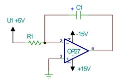
Look at the charging cycle by shorting the capacitor and then removing the short. Is the circuit behaving as you expect?
