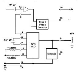
VCO, use an external potentiometer between +5 V and ground, and connect the wiper to pin 9 of the VCO. Look at the output of the VCO at pin 4. As you vary the input to pin 9 over a range from 0 to +5 V, you should see the output frequency of the PLL change. Be sure to write down what frequency range your oscillator range covers.
