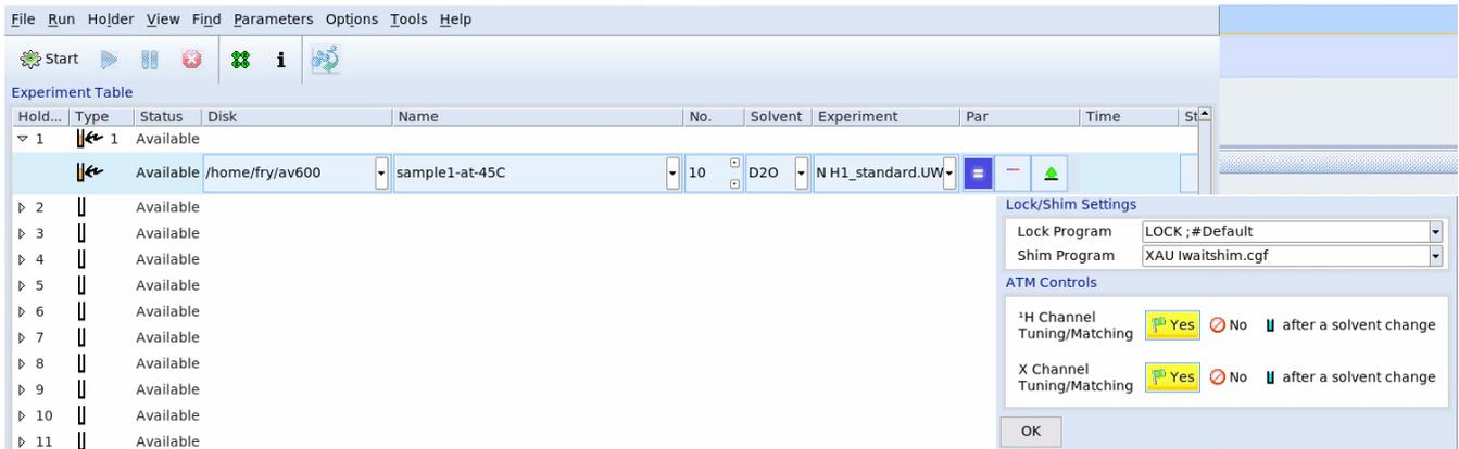
Do the same for all the other samples. Each sample, as it is put in the magnet, will have a delay as set in the automation routine (300 sec in the example above) before shimming will be done.
