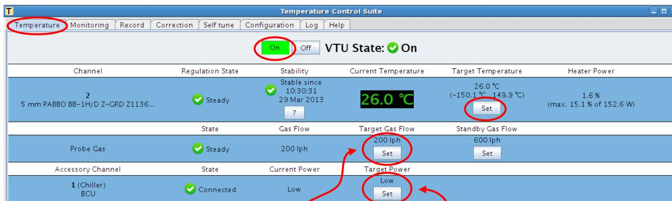
Note the four circled areas. The **Target Gas Flow** and **BCU Target Power** must be set correctly.
