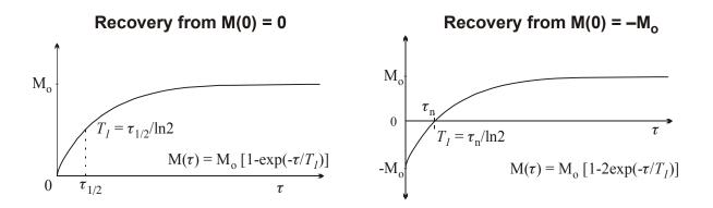
• Usually a quick determination of  $T_I$  is sufficient, allowing proper setting of the repetition delay, **d1**. For most liquids, use the rapid, inversion-recovery method in Section II below. This method involves finding the time at which the magnetization goes through a null,  $\tau_n$ . For more accurate determinations of  $T_I$ , utilize the multi-point fitting scheme described in section III.
